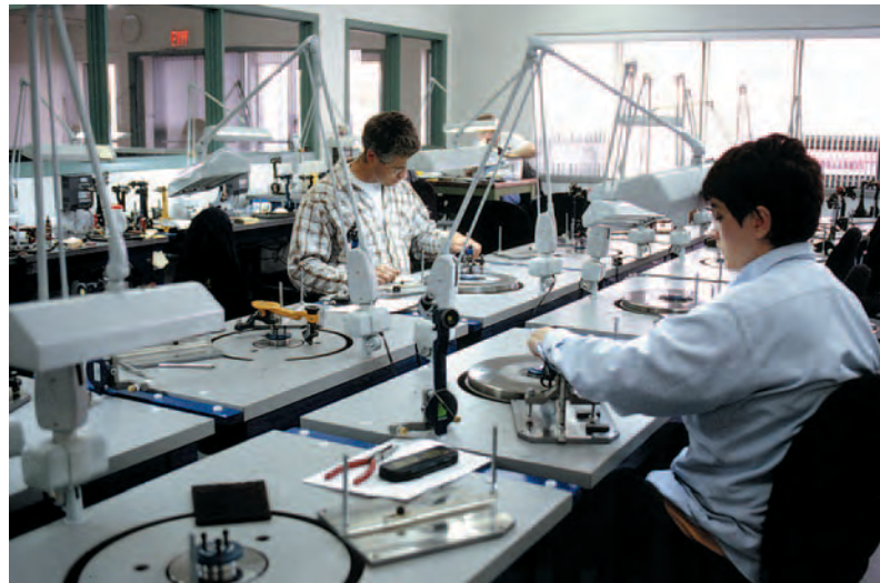
Figure 22. These diamond polishers are working at Sirius Diamonds in Yellowknife, NWT. Sirius was the first cutting facility to open in Canada’s Far North, to manufacture diamonds from the Ekati mine. Photo © Tim Atherton, 2000.
