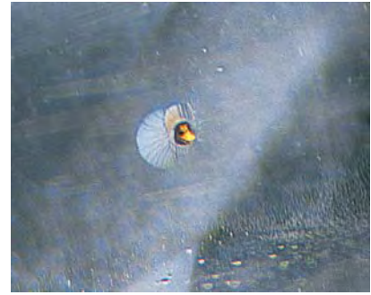
Figure 5. Also present in all of the faceted bromellites were several transparent rounded yellow crystals surrounded by haloes. Magnified 40x.
