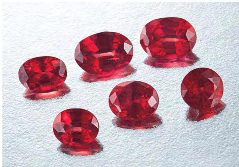
Figure 1. These strongly saturated red stones were marketed as "Diffusion Ruby." However, gemological testing revealed that they are actually the result of a synthetic ruby overgrowth onto colorless to near-colorless natural sapphire. These six samples (0.80–1.12 ct) are part of the group studied in detail for this report. Photo by Maha Tannous.
