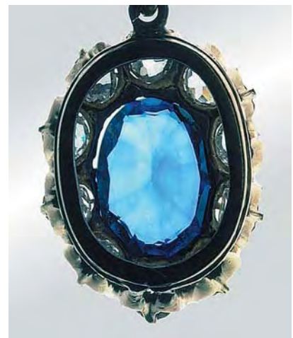
Figure 16. As seen with immersion and the earring viewed from the back, the shallow and patchy blue coloration, plus the “outlining” of the facet junctions, serves as proof that the blue color in the synthetic sapphire was produced by bulk diffusion.
